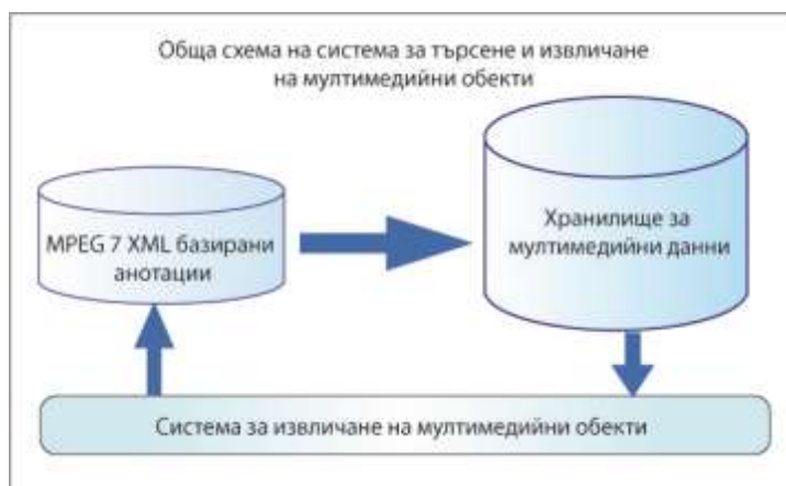
Figure 3. General scheme of a system for searching and retrieving multimedia objects from MPEG-7 based storage
